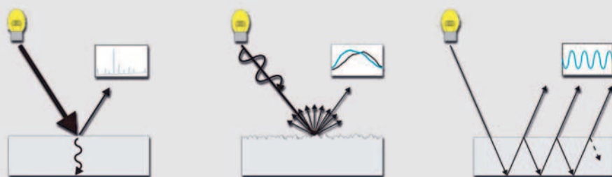
Figure 2: a) Absorption/reflection can determine composition; b) Surface effects can determine surface roughness and grain size; c) Interface effects can determine layer thickness.
